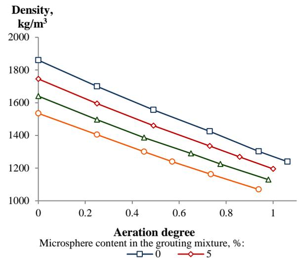
**Figure 2.** Dependence of the density of the mixtures to the degree of the aeration and the content of HASM
