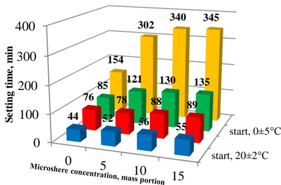
**Figure 1.** Dependence of setting time of backfill mixes content in their composition, and SAHM ambient temperature
