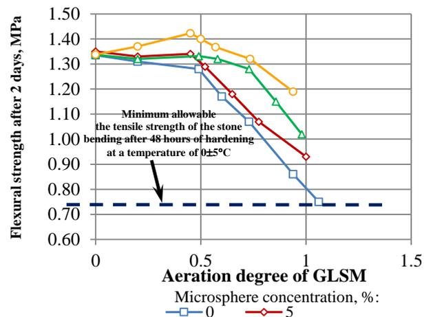
**Figure 5.** Dependence of the strength of cement the degree of aeration of the cement mixture and the content of hollow microspheres
