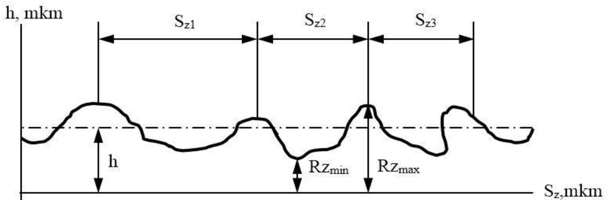
**Figure 2.** Deposit relief microstructure on rotor blades of the first stage ( $\times 240$ )
