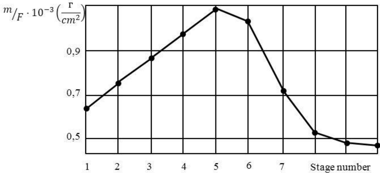
**Figure 1.** The distribution of deposit mass on the rotor blades on the compressor stages
