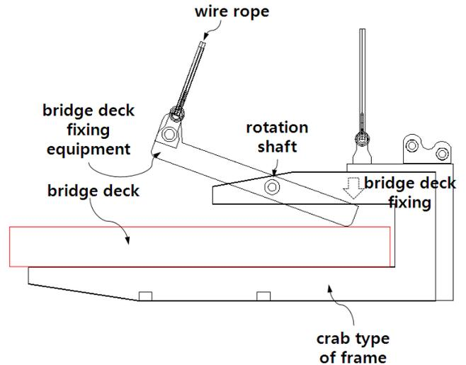
**Figure 4.** Development of new lifting technique for concrete bridge decks
