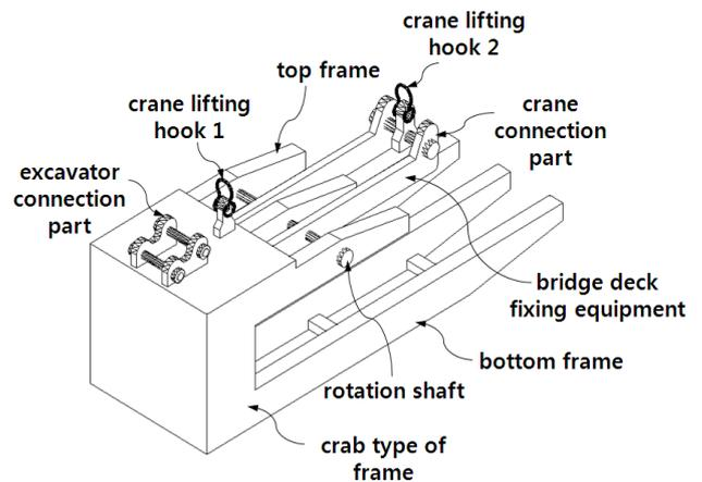
**Figure 2.** Development of new lifting technique for concrete bridge decks
