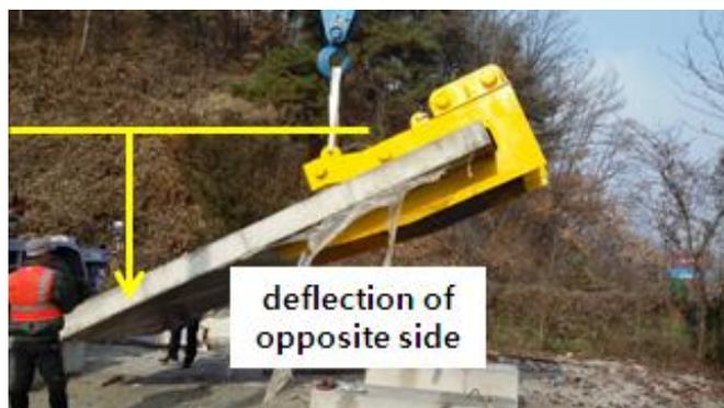
Figure 7. Test scene of concrete lifting using a crane
