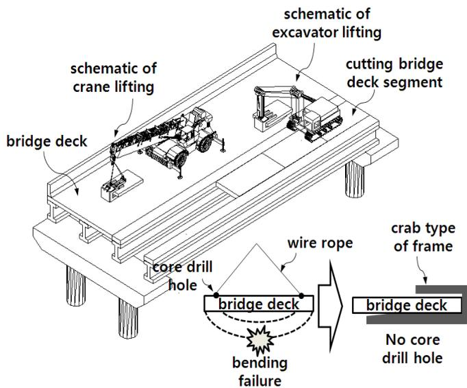
**Figure 3** Development of new lifting technology for concrete bridge deck
