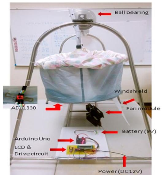
Figure 2. Automatic Rocking Based cradle
