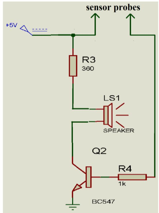
Figure -3. Wet Sensor based cradle circuit diagram
