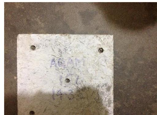
**Figure 5.** FCB with 10% and 15% fiber content showed efficient drilling characteristics
