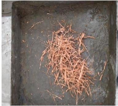
**Figure 2.** Coconut Fibers after separation
