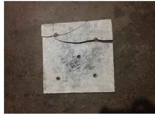
**Figure 4.** FCB with 5% fiber content experienced cracks and detachment
