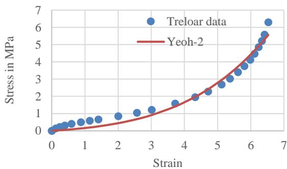
**Figure 4:** Curve fitting data for Yeoh-2order
