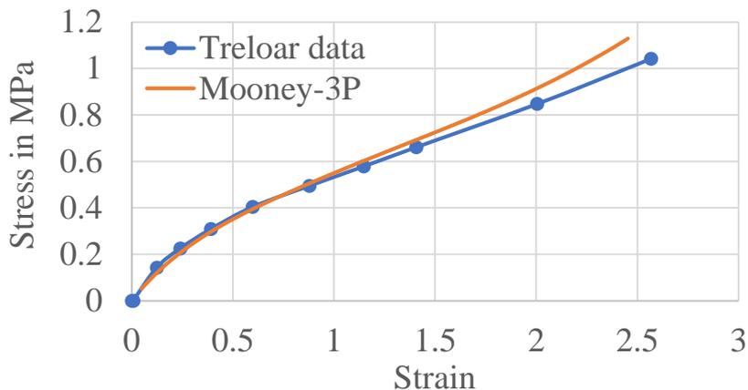
**Figure 7:** Comparison of Mooney-3P stress-strain curve with Treloar's Data
