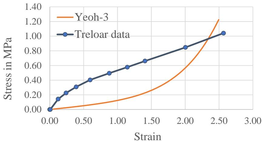
**Figure 10:** Comparison of Yeoh-3 order stress-strain curve with Treloar's Data
