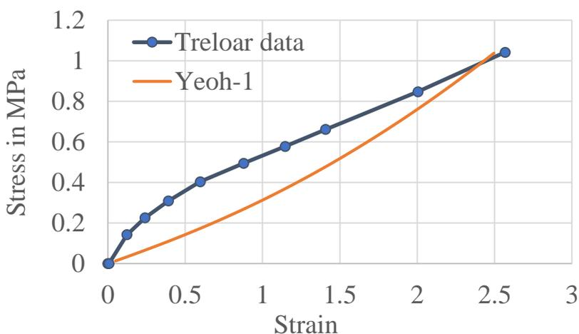
**Figure 8:** Comparison of Yeoh-1 order stress-strain curve with Treloar's Data
