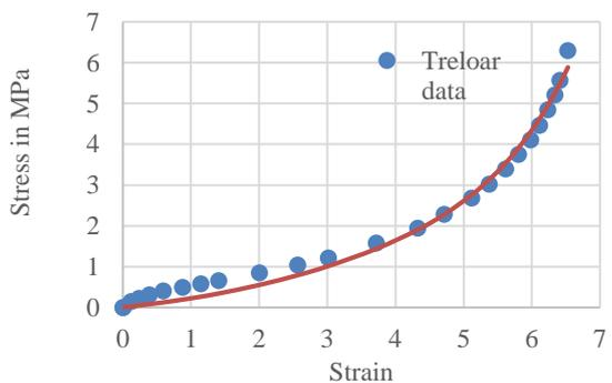
**Figure 5:** Curve fitting data for Yeoh-3order
