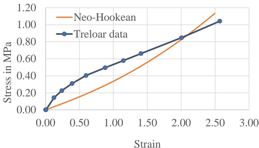
**Figure 11:** Comparison of Neo-Hookean stress-strain curve with Treloar's Data
