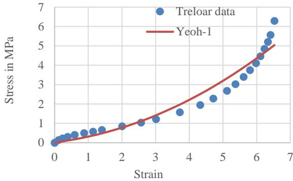
**Figure 3:** Curve fitting data for Yeoh-1order
