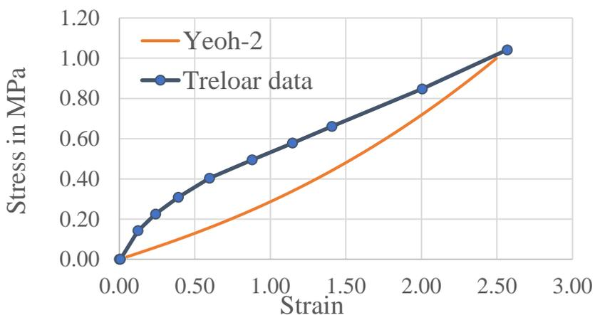
**Figure 9:** Comparison of Yeoh-2 order stress-strain curve with Treloar's Data
