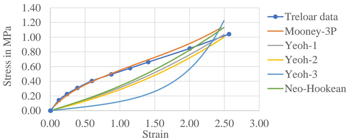
**Figure 12:** Comparison of all respective model's stress-strain curves with Treloar's Data
