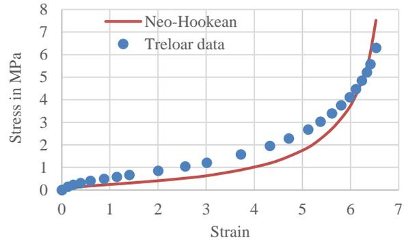
**Figure 6:** Curve fitting data for Neo-Hookean model
