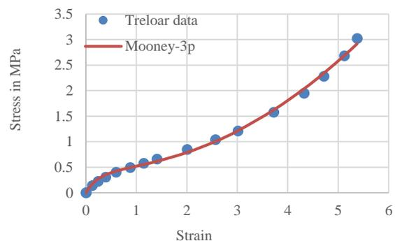
**Figure 2.** Curve fitting data for Mooney-3parameter
