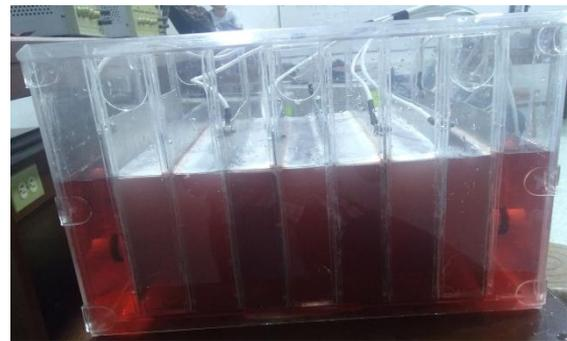
**Figure 2.** Implementation of electroflocculation system
