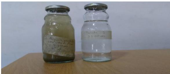
**Figure 4.** Inlet water without treatment and outlet water treated by electrostatic flocculation
