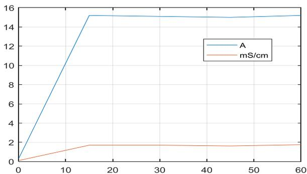
**Figure 8.** Behaviour of the electrical conductivity in the electroflocculation process
