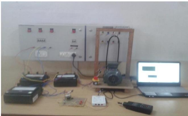
Figure 5. Experimental Setup for Stator Winding Short Circuit Fault Detection
