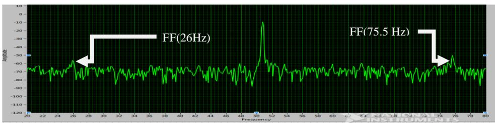
**Figure 8.** Power spectrum of healthy motor with 23 % shortened under no load condition
