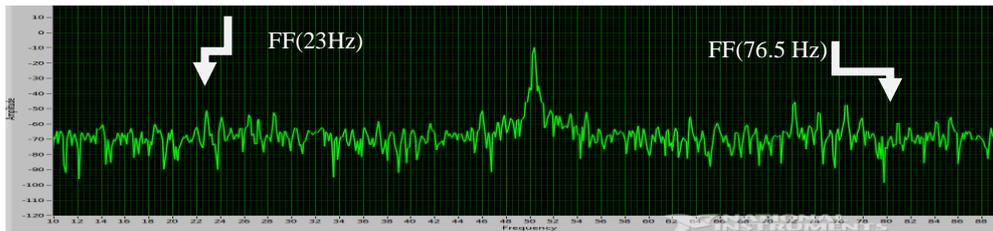
Figure 11. Power spectrum of healthy motor with 23 % shorted under full load condition
