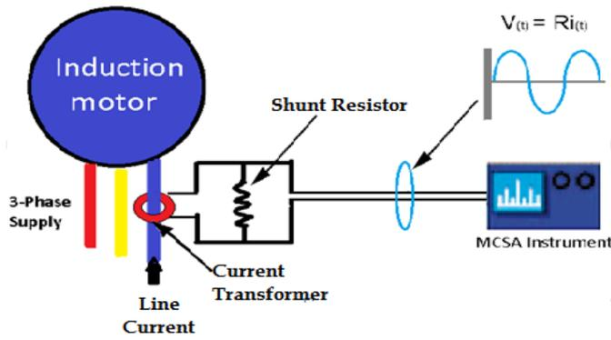
Figure 4. Basic MCSA Instrumentation Diagram
