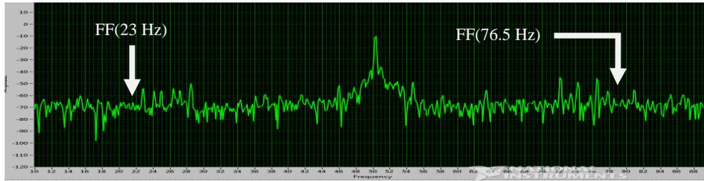
Figure 10. Power spectrum of healthy motor with 7.5 % shorted under full load condition
