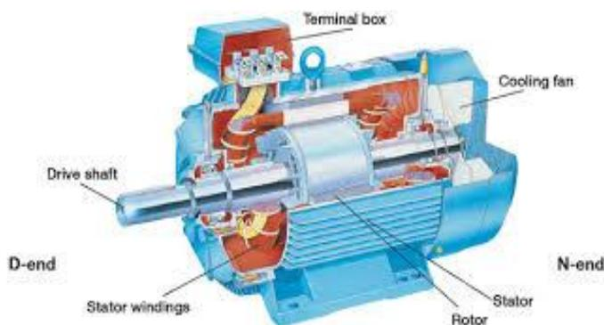
Figure 2. General diagram of induction motor
