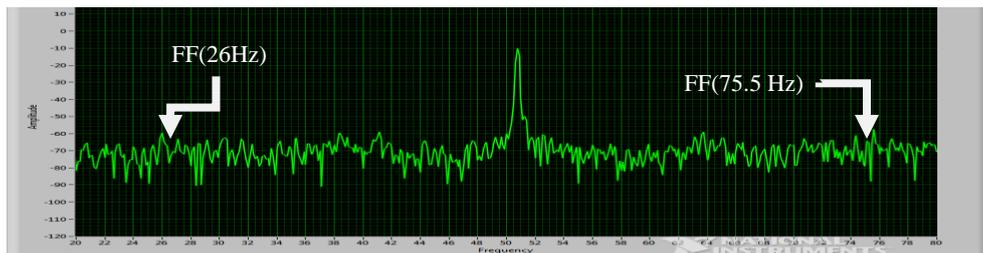
**Figure 7.** Power spectrum of healthy motor with 7.5 % shorten end under no load condition
