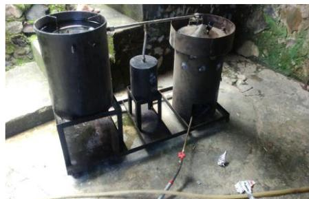
**Figure 1.** Model of pyrolysis apparatus used for carbonizing the salak seed and coconut shell
