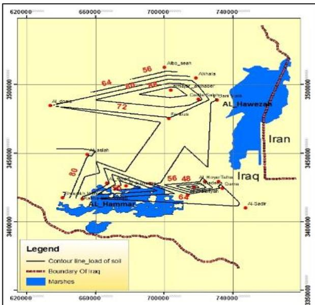
Figure 3. Contour map showing the values of bearing capacity in marshes soil
