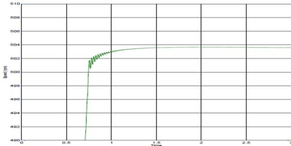
**Figure 4.** Speed obtained by SMO based MRAS method
