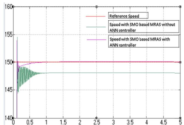
**Figure 10.** Speed estimation obtained from SMO based MRAS with and without ANN controller
