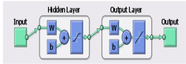
Fig.2: A two-layer feed-forward network with sigmoid hidden neurons and linear output neurons
