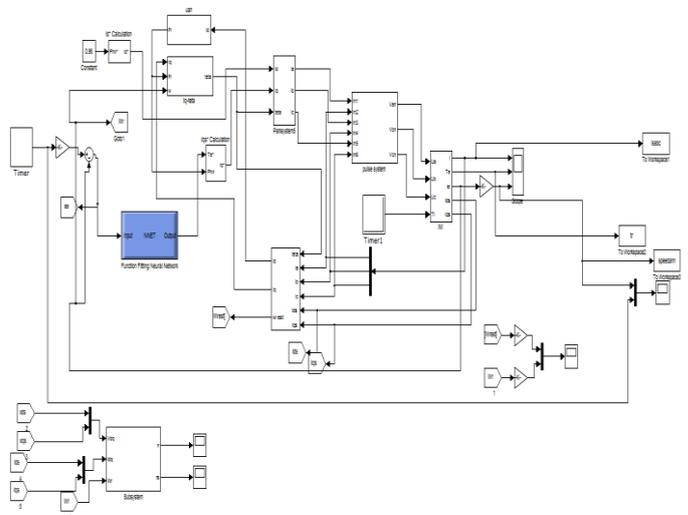
Figure 3. SMO based MRAS with ANN controller based Induction motor drive
