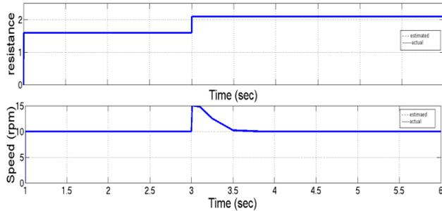
**Figure 11.** Speed Estimation and Stator Resistance Identification at Speed Command of 10 rpm and Sharp Variation of Stator Resistance.
