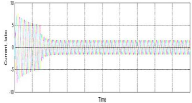
**Figure 8.** Current waveform obtained by SMO based MRAS with ANN controller
