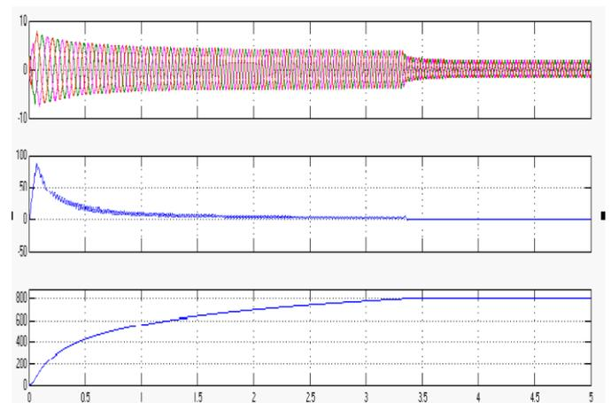
**Figure 15.** (a) Current, (b) Torque and (c) Speed waveforms
