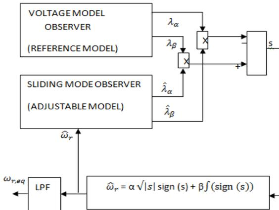
Figure 1. Block diagram of second order SM MRAS speed estimator
