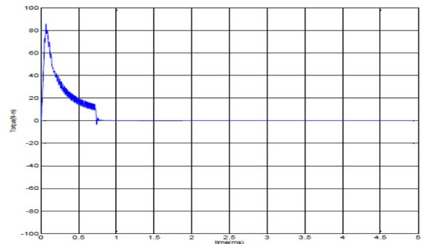
**Figure 9.** Torque waveform due to SMO based MRAS with ANN controller
