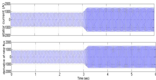
**Figure 12.** Stator current and rotor flux waveforms
