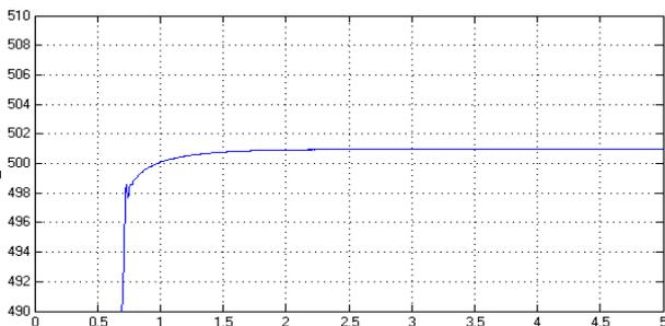
**Figure 7.** Speed estimation obtained from SMO based MRAS with ANN controller
