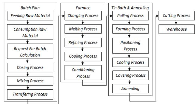
Figure 1.2 Flow of Glass Making Process
