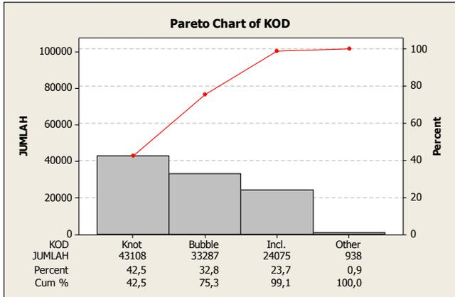
Figure 4.3 Pareto Diagram of glass defects
