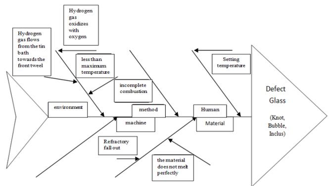
Figure 4.5 Fishbone diagram for glass defects
