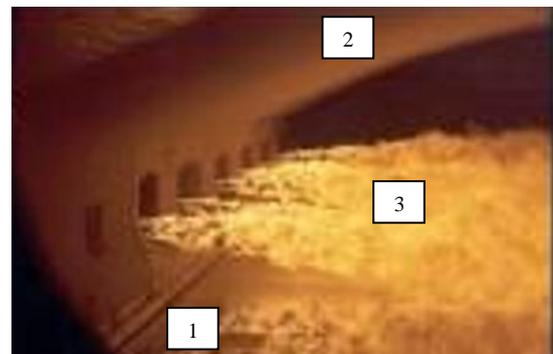
Figure 1.3 Combustion in the furnace: 1: Molten Glass; 2: Crown; 3: Flame
