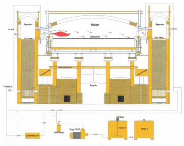
**Figure 4.7** Flow Process TNBT
