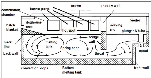
Figure 2.1 Section in a furnace [4]
