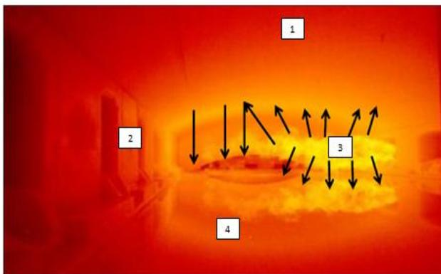
Figure 2.2 The inside of the furnace: 1: Crown; 2: sidewall; 3: Fire burning; 4: Molten Glass [4]
