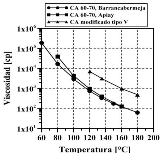
Fig. 1. Viscosity curve of the analyzed asphalts
