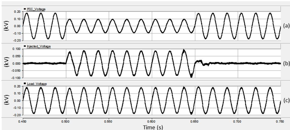
**Fig. 12.** Result showing voltage sag. (a) PCC voltage. (b) Compensation voltage. (c) Load voltage.
