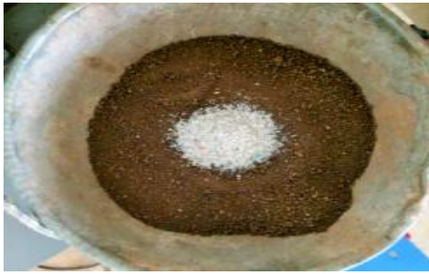
Figure 2: shows black cotton soil with waste PET bottles
