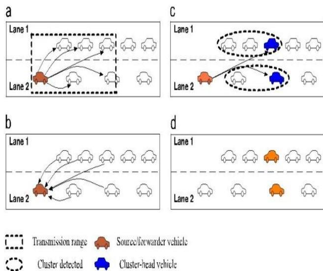
**Figure 3.3** Main phases of SRB technique: (a) RTB transmission, (b) CTB transmission, (c) Cluster detection and CH election, and (d) message propagation.
