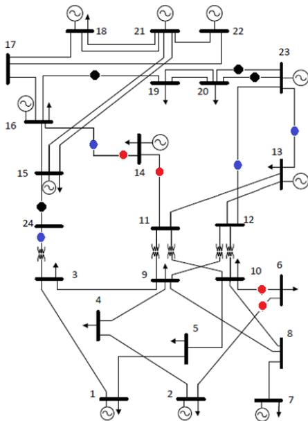
**Figure 4.** Illustration of interdiction plans for different load profiles: high (blue dots), medium (black dots) and low (red dots).
