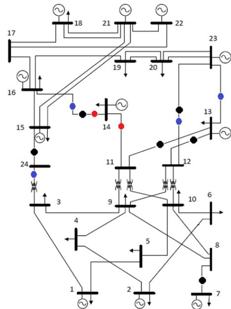
**Figure 3.** Illustration of interdiction plans for  $M=2$  (red dots),  $M=4$  (blue dots), and  $M=6$  (black dots).
