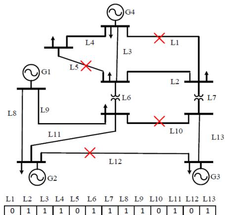
Figure 1. Illustration of an interdiction vector in a power system.
