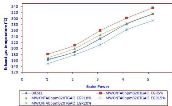
Fig. 8 Exhaust gas against Brake Power
