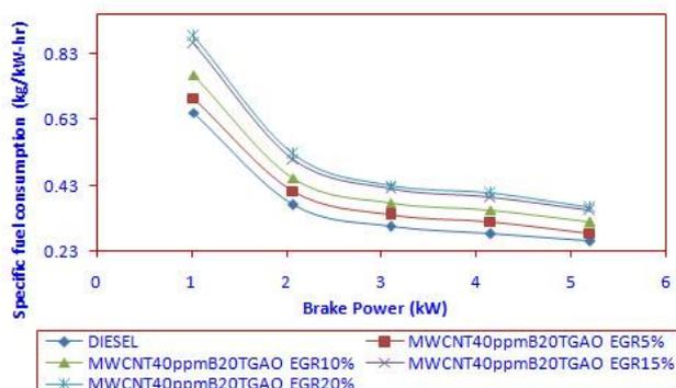
**Fig.2** Specific fuel consumption against Brake power
