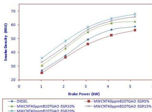
**Fig.4** Smoke density against Brake Power
