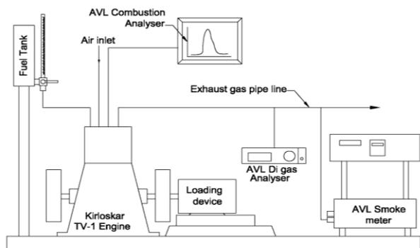
**Fig.1** Experimental arrangement
