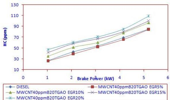
Fig. 6 Hydrocarbon against Brake Power
