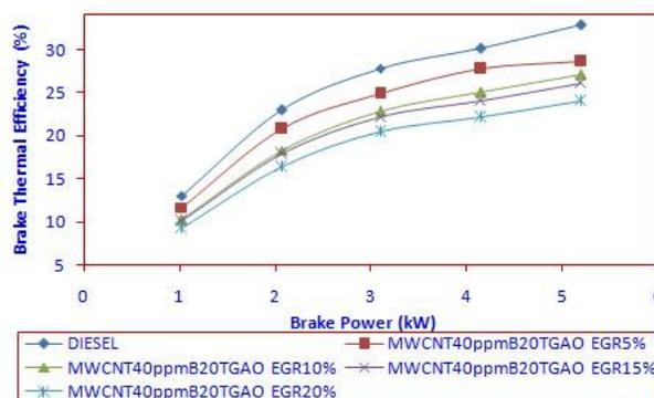
**Fig.3** Brake thermal efficiency against Brake power
