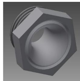
**Figure 5.** CAD model of hollow cone nozzle with geometry modification.
