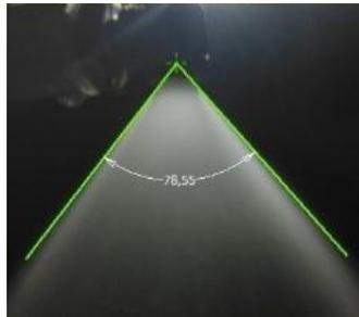
**Figure 14.** Spray angle straight nozzle experimental test.
