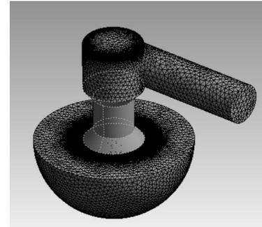
**Figure 4.** Meshing of the control volume of the cup-straight nozzle assembly and injection chamber.
