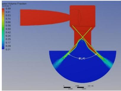
**Figure 7.** Contours of volumetric fraction in plane of symmetry of the straight nozzle sprinkler.
