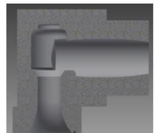
**Figure 6.** CAD model of spiral distributor with geometry modification.
