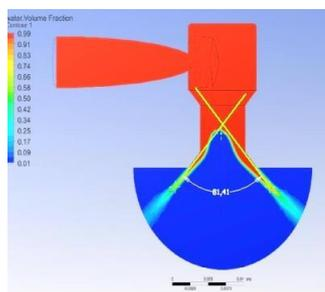
**Figure 13.** Spray angle straight nozzle CFD simulation.
