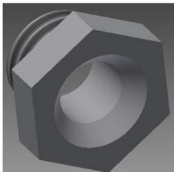
**Figure 3.** CAD model of straight studio nozzle.
