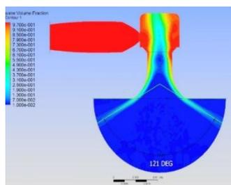
**Figure 15.** Spray angle hollow cone nozzle CFD simulation.
