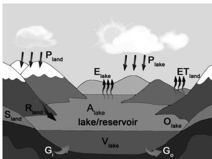
Figure 4. The general water-balance components for a lake or reservoir and its surrounding catchments
