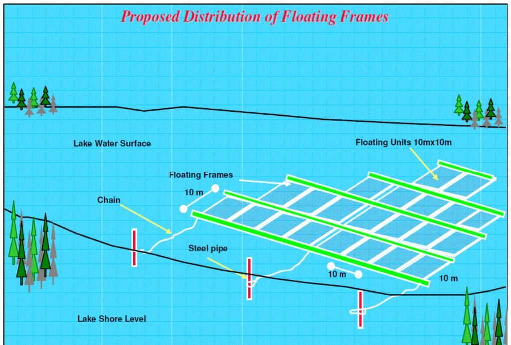
**Figure 10.** The proposed distribution of floating frames (Pontoon) on the lake surface
