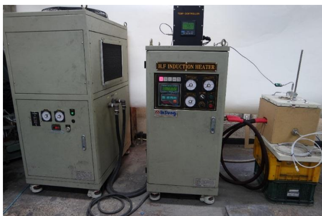
Figure 2. Experimental apparatus for removal and recovery of arsenic from gold concentrate.
