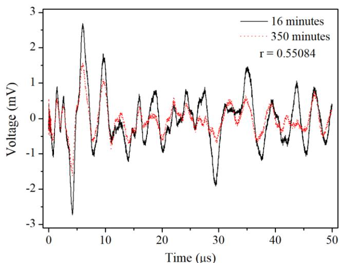
**Figure 3.** Comparison between the photoacoustic signals obtained at 16 minutes and 350 minutes after the synthesis. When comparing the photoacoustic signals was obtained the correlation coefficient of 0.55084.
