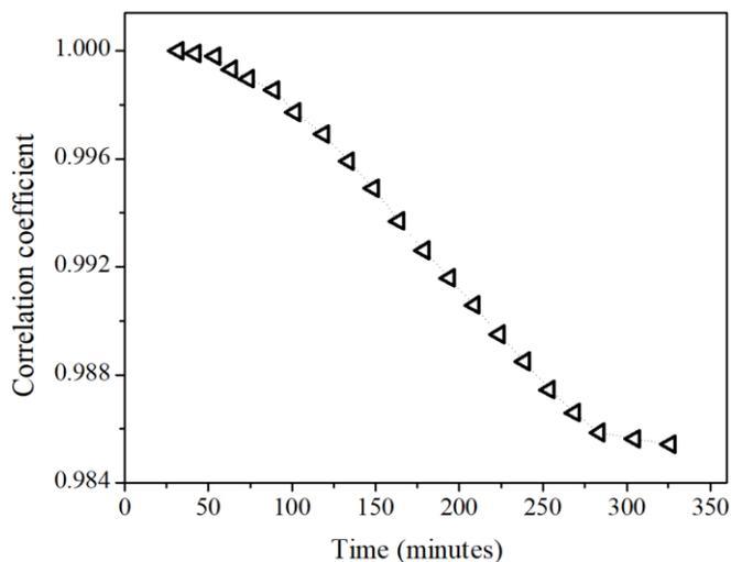
**Figure 8.** Correlation coefficient as a function of the time elapsed after the synthesis. The first absorption spectrum obtained at 32 minutes after the synthesis was correlated with all spectra.
