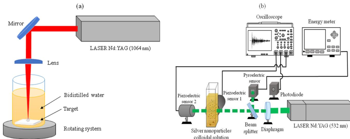
**Figure 1.** Schematic representation of experimental setups: (a) experimental setup used to realize the synthesis of silver nanoparticles by laser ablation of a silver target submerged in bidistilled water, (b) experimental setup used to study changes in optical properties of silver nanoparticles colloidal solution by pulsed photoacoustic and transmittance techniques.
