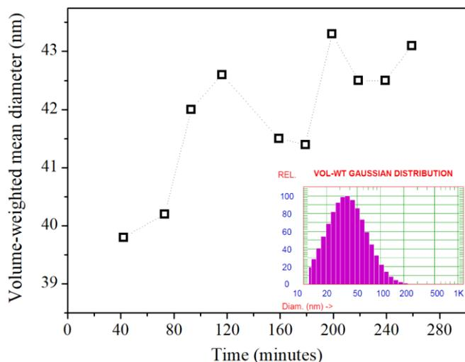
**Figure 9.** Hydrodynamic size of the silver nanoparticles as a function of the time elapsed after the synthesis. Inset shows volume weighted size distribution of silver nanoparticles for 259 minutes after the synthesis.
