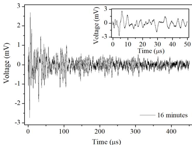
**Figure 2.** Photoacoustic signal of colloid with silver nanoparticles in bidistilled water. This signal was obtained at 16 minutes after the synthesis. The inset shows the time evolution during the first 50  $\mu$ s.
