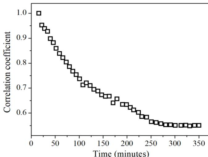
**Figure 4.** Correlation coefficient as a function of the time elapsed after the synthesis. It was correlated the signal obtained at 16 minutes after the synthesis with all the signals.
