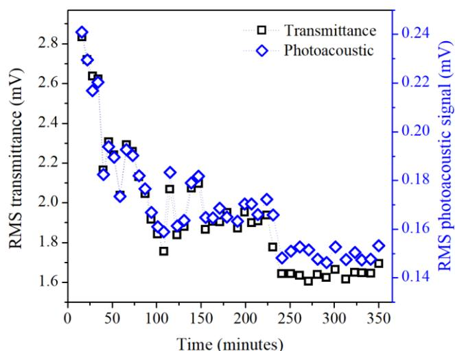
**Figure 5.** RMS and Transmittance of the photoacoustic signal of the colloid as a function of the time elapsed after the synthesis.
