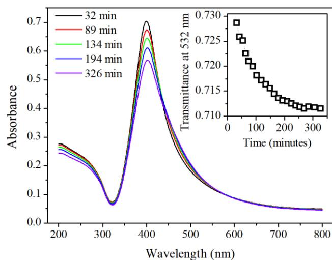
**Figure 6.** Absorption spectrum of colloid with silver nanoparticles as a function of the time elapsed after the synthesis. The inset shows the transmittance of colloid at 532 nm as a function of time.
