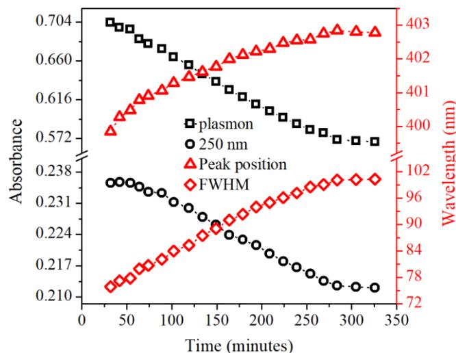
**Figure 7.** Absorbance of the surface plasmon ( $\square$ ), absorbance at 250 nm ( $\circ$ ), position of the surface plasmon ( $\Delta$ ) and width at half height of the band corresponding to surface plasmon (FWHM) ( $\diamond$ ) as a function of the time elapsed after synthesis.
