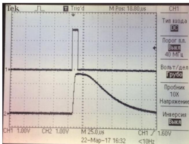
**Figure 7.** Protracted trailing edge of the pulse at the output of the phototransistor.
