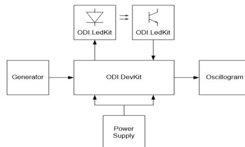
Figure 1 - Connection diagram of the test setup.
