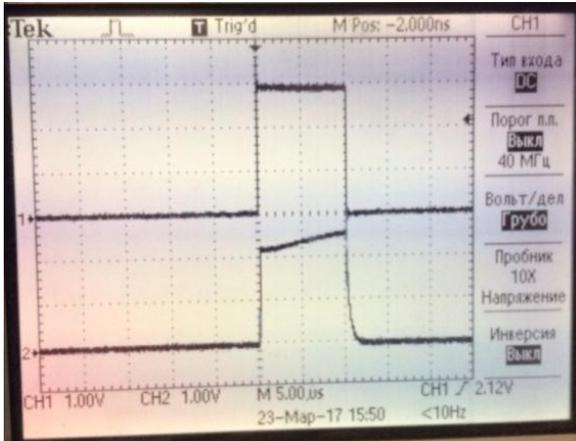
**Figure 8.** Signal on the emitter and the output of the receiver while controlling the power of the phototransistor.
