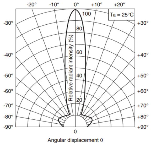
Figure 4 – Radiation Diagram GL100MN1MP
