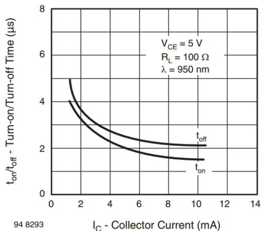
**Figure 6** – Response time of the TEMT1000 photodetector from the collector current
