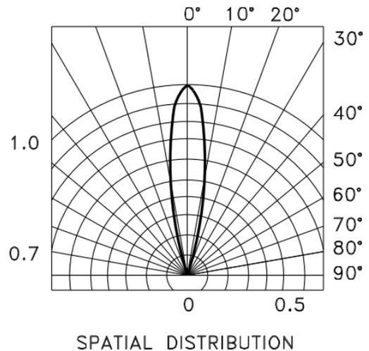
Figure 5 – Radiation Diagram KM2520SF4C03
