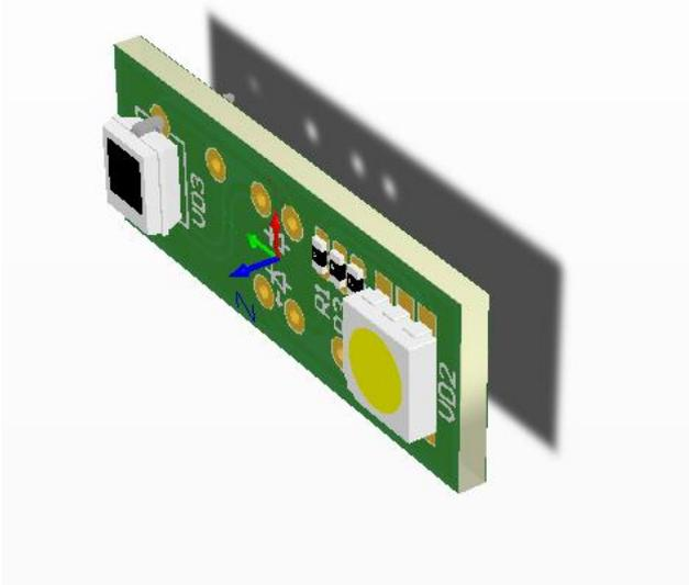
Figure 3- circuit board set of the debugging layout
