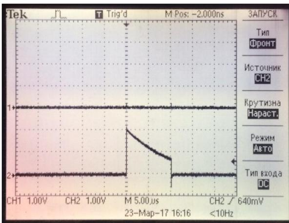
**Figure 9.** The signal at the output of the phototransistor when the power is switched (there is no emitter signal)
