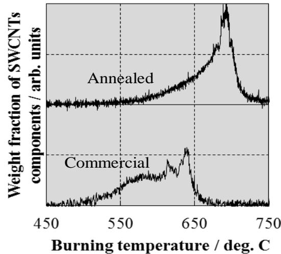
**Figure 3.** First derivative thermogravimetric curves of the commercial and annealed single-walled carbon nanotubes measured under an air atmosphere.
