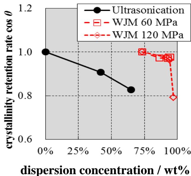
**Figure 4.** Dispersion concentration vs. crystallinity retention rate for highly crystalline single-walled carbon nanotubes dispersed by ultra-sonication and wet-jet milling. Ultra-sonication at 40 kHz was performed for 0, 5 and 10 h. Wet-jet milling was operated at both 60 and 120 MPa and repeated 1, 3, 5 and 10 times.
