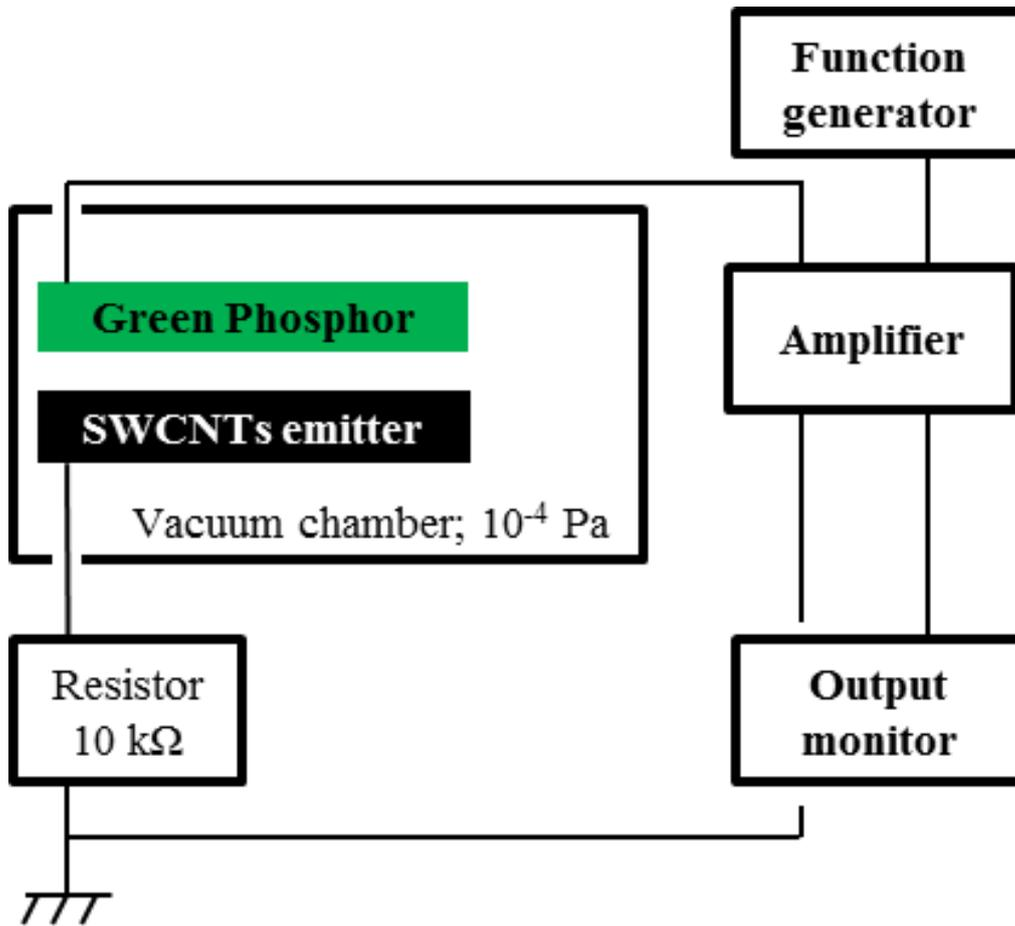
**Figure 1.** Schematic diagram of the current–voltage measurement system. A pulse wave with a duty cycle of 4 % at a frequency of 60 Hz was applied.
