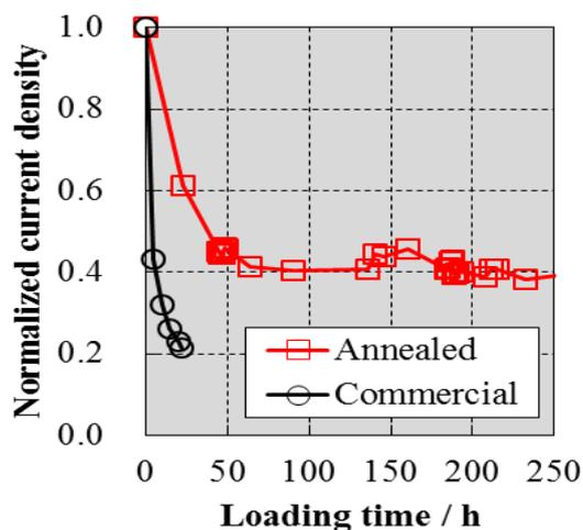
**Figure 6.** Field emission stability of highly crystalline single-walled carbon nanotube and commercial single-walled carbon nanotube emitters measured at 7 V/ $\mu\text{m}$ . Both emitters used SWCNT inks that were prepared by wet-jet milling at 120 MPa for 5 cycles.
