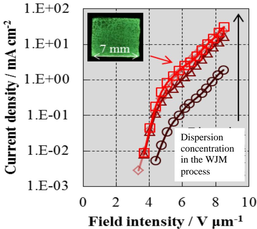
**Figure 5.** I-V plots of field emitters prepared using highly crystalline single-walled carbon nanotube inks dispersed by 1-10 wet-jet milling cycles at 120 MPa. The inset shows a luminescence photograph of 5 wet-jet milling cycles.
