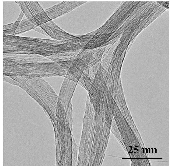
**Figure 2.** Transition electron micrograph of the annealed single-walled carbon nanotubes.
