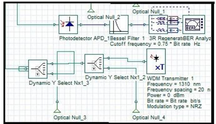
Figure 9. Upstream layout of TDMA
