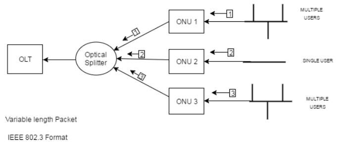
**Figure 2.** Upstream principle in EPON
