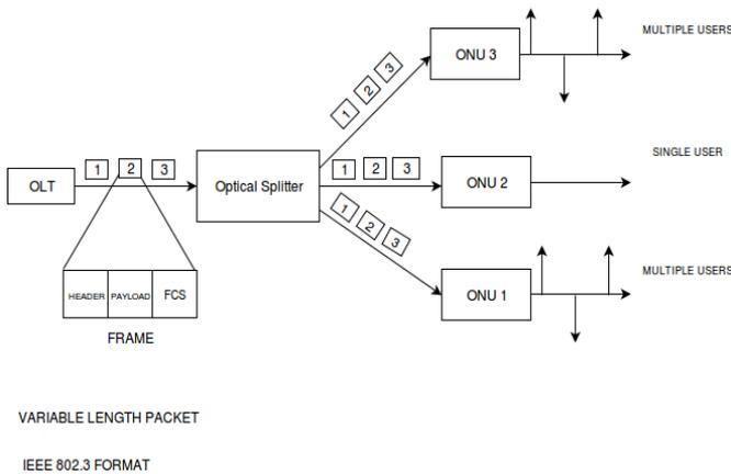
**Figure 1.** Downstream principle in EPON
