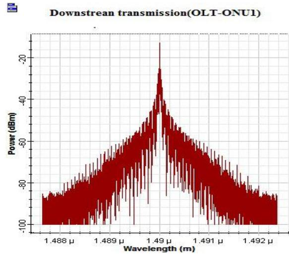
Figure 4. Downstream spectrum into the first optical fiber
