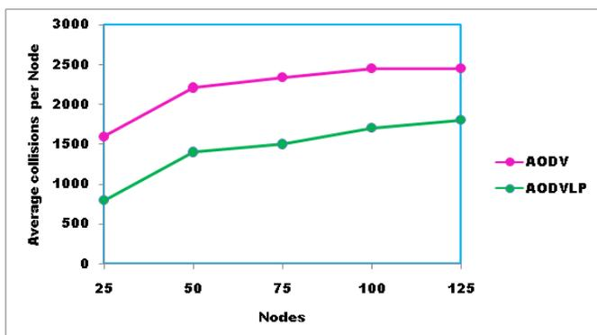
Figure 4. Response of response of RTS collisions per node at CBR using AODV and AODVLP
