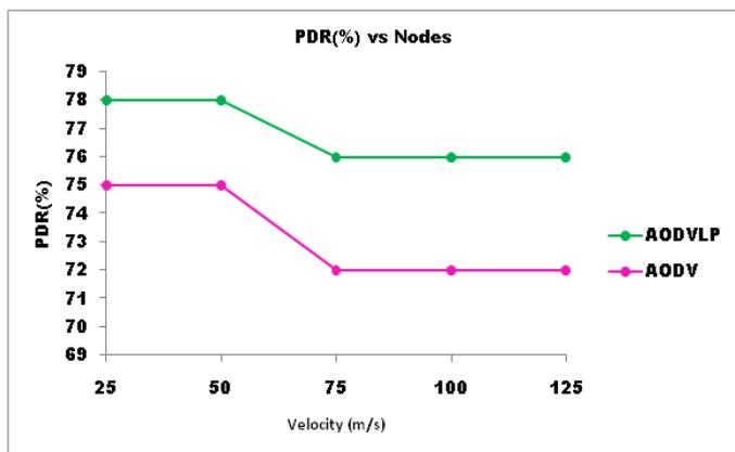
**Figure 7.** Response of packet delivery ratio with respective velocity at CBR using AODV and AODVLP
