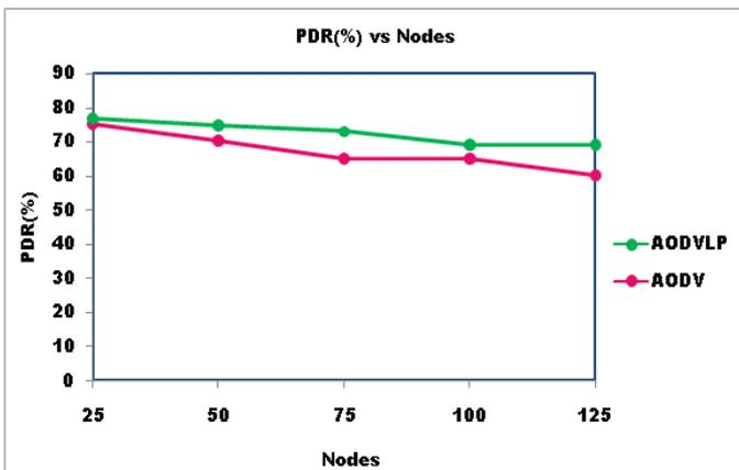
Figure 3. Response of packet delivery ratio at CBR using AODV and AODVLP
