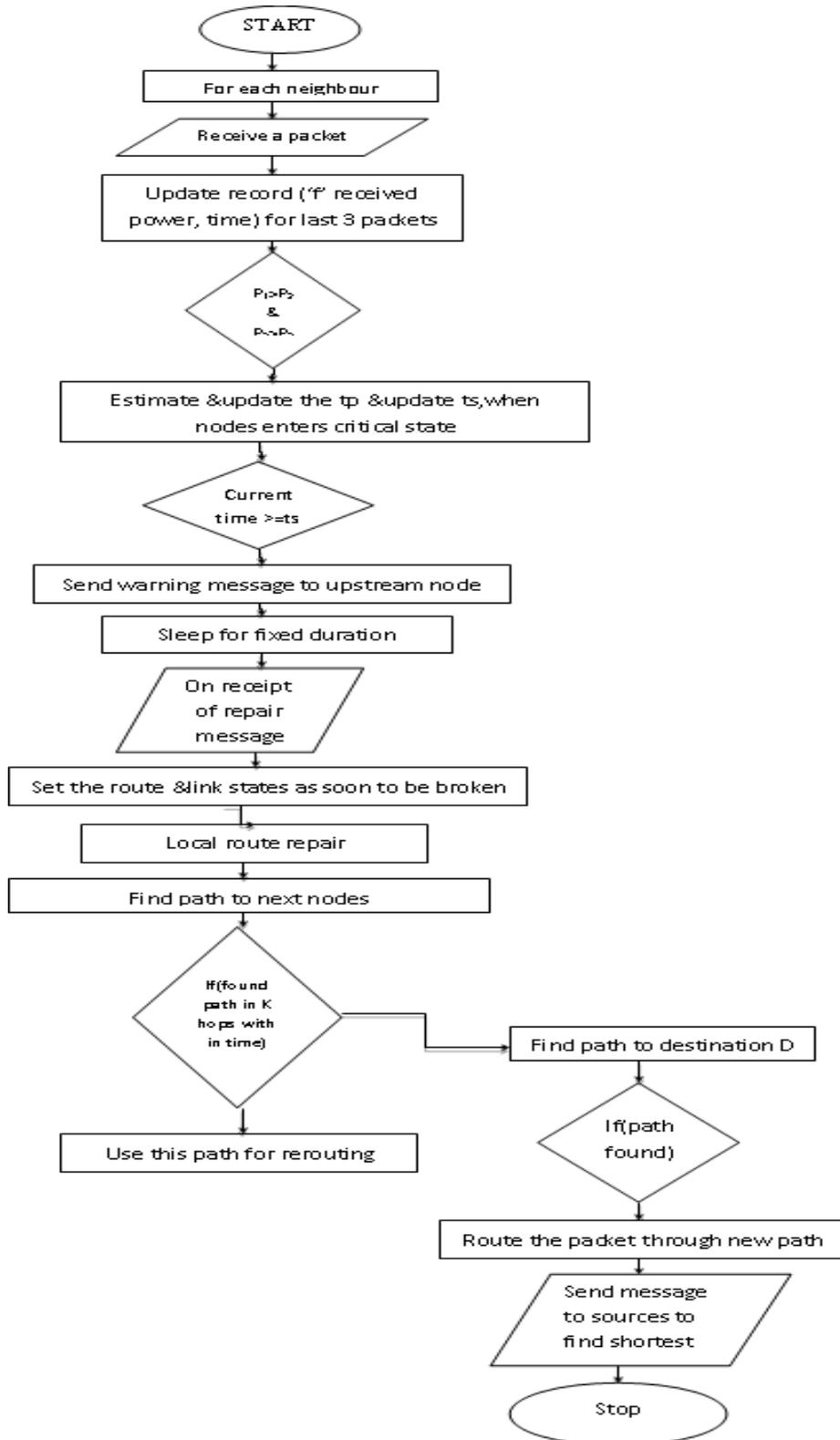
Figure 1. Flowchart of link prediction algorithm
