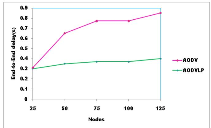
Figure 5. Response of RTS end-to-end delay at CBR using AODV and AODVLP
