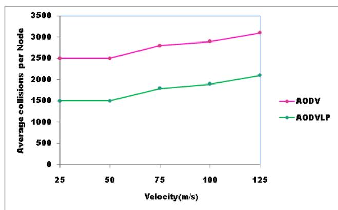
**Figure 8.** Response of RTS collisions with respective velocity at CBR using AODV and AODVLP
