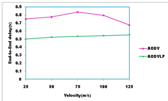
**Figure 9.** Response of end-to-end delay with respective velocity at CBR using AODV and AODVLP
