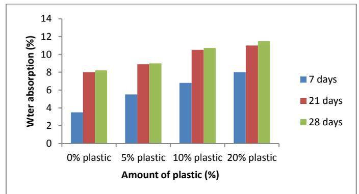
**Figure 2.** Water absorption of the specimens containing plastic aggregate (MB Hossain et al., 2016)
