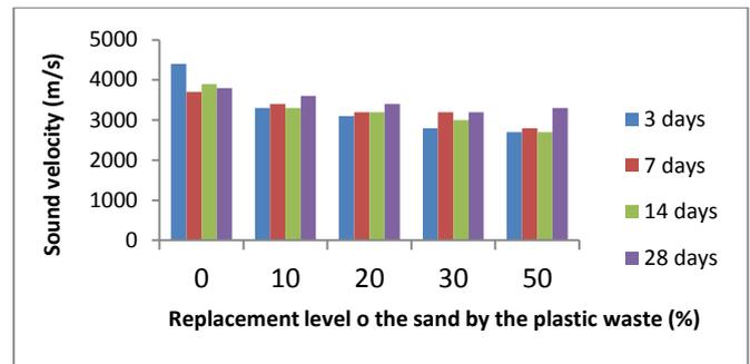
**Figure 1.** Evolution of the sound velocity of self-compacting mortars as function of curing time (3, 7, 14 and 28) days (Brahim Safi et al., 2013)
