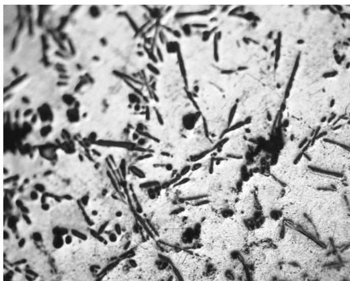
**Figure 1:** Optical microstructure of Al-1wt. %Mg-10 wt.% SiC
