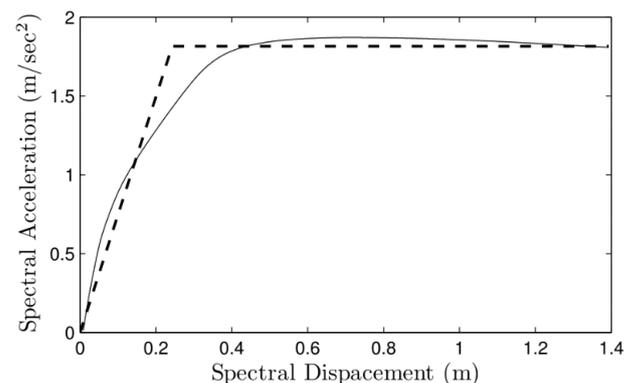
Fig. 5: Capacity Spectrum of the equivalent *SDOF* system (longitudinal direction).
