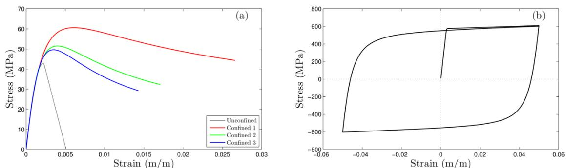
Fig. 4: Constitutive laws used to model the behavior of the materials: (a) Monotonic behavior for the cover and the confined cores' concrete material; (b) Cyclic behavior of the reinforcing steel material.
