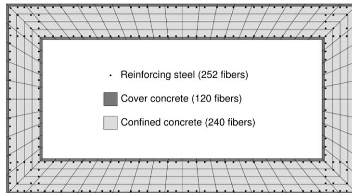
Fig. 3: Typical fiber section of the piers.
