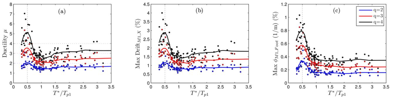
**Fig. 9:** Maximum response quantities of the structure for the three intensity levels: (a) Ductility of the equivalent *SDOF*; (b) Maximum drift of Pier M1; (c) Maximum Curvature at the base of pier M1. Solid lines correspond to the moving average of the obtained data.
