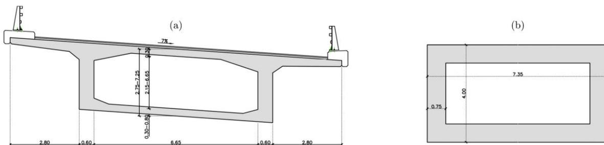
Fig. 2: Typical cross sections (a) Deck, (b) Piers.
