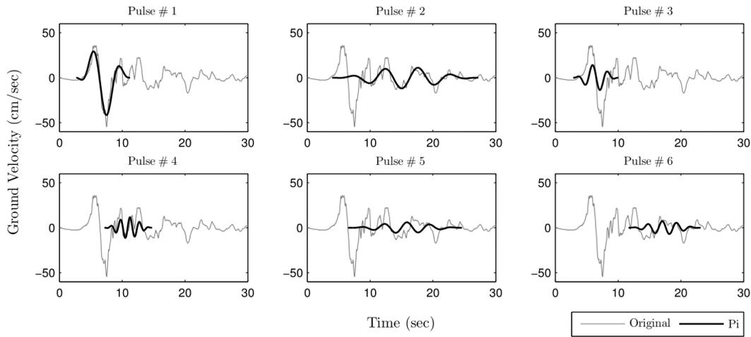
**Fig. 7:** Velocity time histories of the first six significant pulses (bolded lines) for the EC County FF station record of the Imperial Valley, 1979 Earthquake. The original record is shown with grey line.
