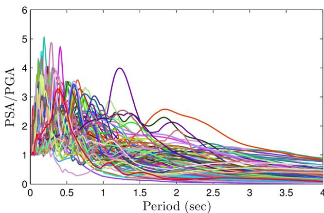
**Fig. 6:** Elastic Pseudo-Acceleration response spectra for 5% damping of the considered records, normalized with respect to their *PGA*.
