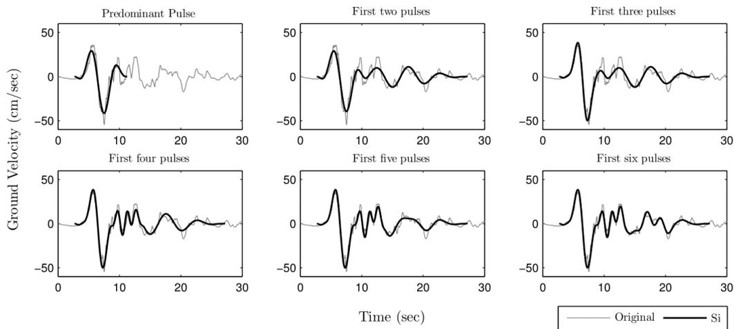
**Fig. 8:** Velocity time histories of the six corresponding pulse records (bolded lines) for the EC County FF station record of the Imperial Valley, 1979 Earthquake. The original record is shown with grey line.
