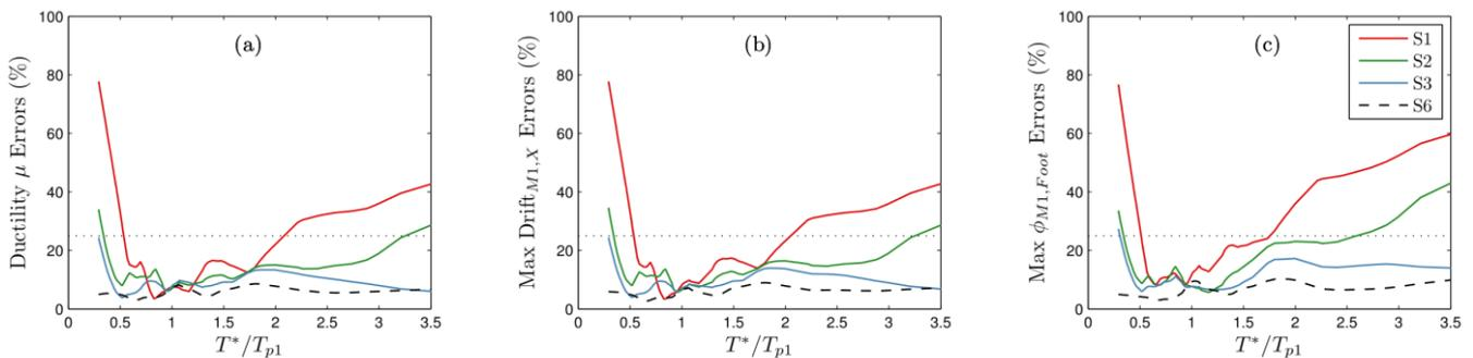
**Fig. 10:** Moving averages of the absolute values of the errors produced using pulse records  $S_1, S_2, S_3$  and  $S_6$  for  $q_y = 4$ : (a) Ductility of the equivalent *SDOF*; (b) Maximum drift of pier M1; (c) Maximum curvature at the base of pier M1.
