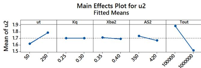
Figure 5. Main effects plot for optimum gear ratio of helical gear unit
