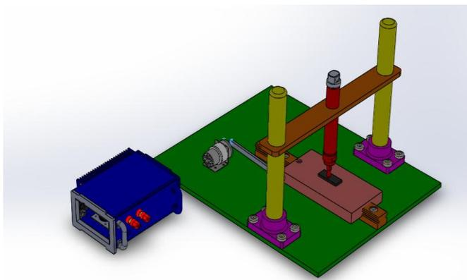
**Fig.1:** Schematic diagram of the reciprocating tester (ASTM G133)
