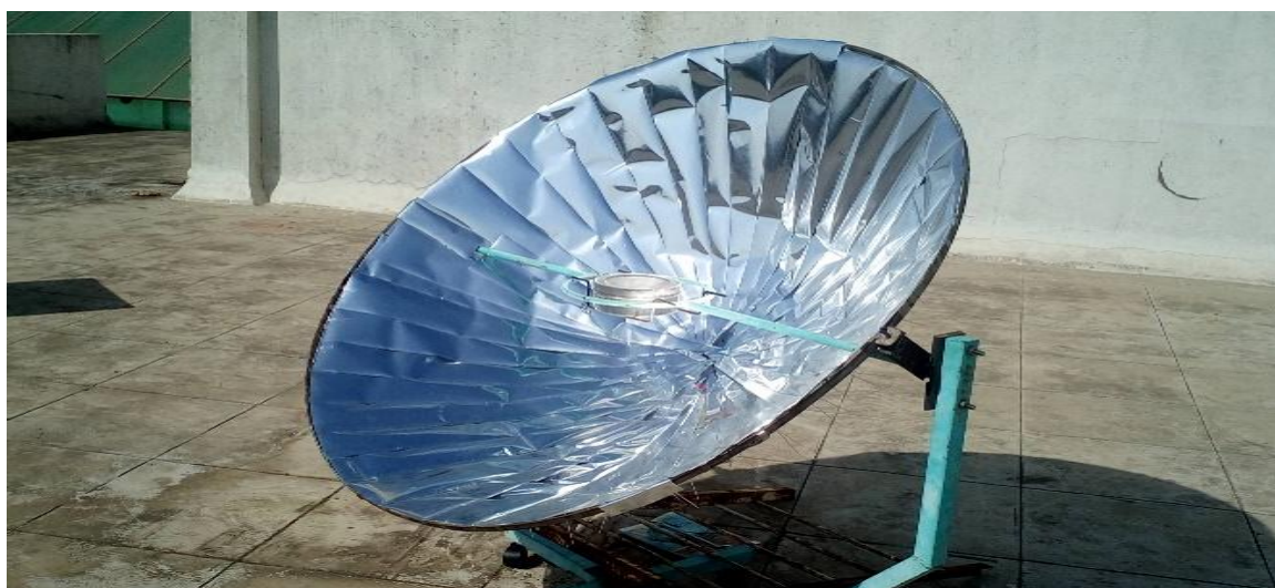
Figure 4. Parabolic Dish Collector with Aluminum Polymer Fil
