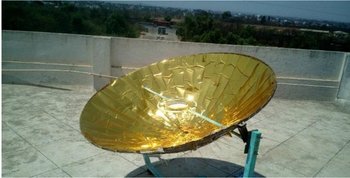
Figure 5. Parabolic Dish Collector with Gold Chrome Polymer Film
