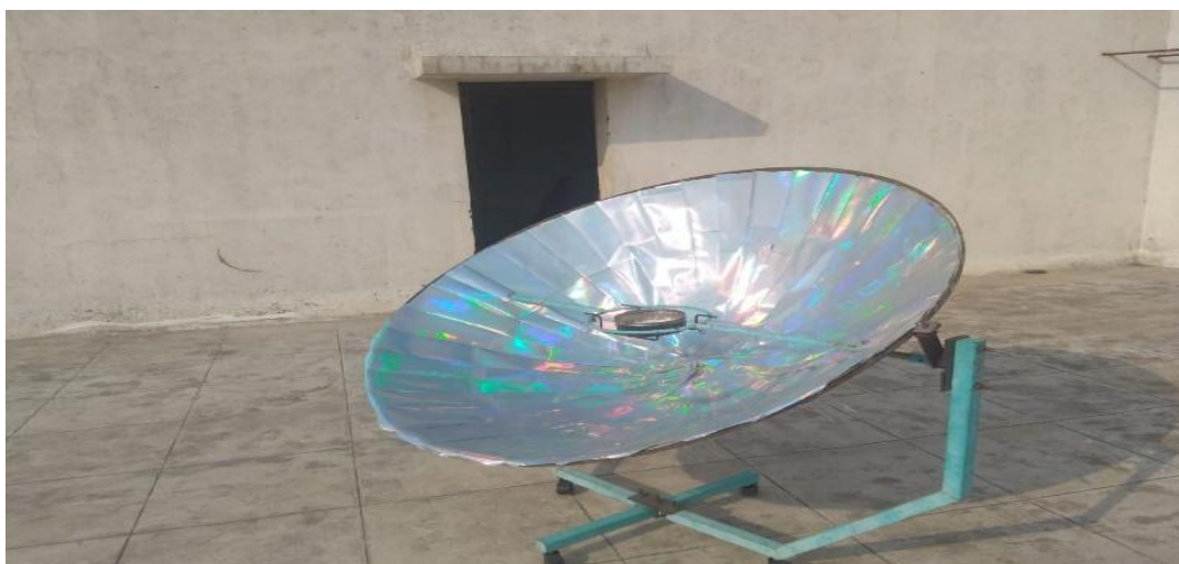
Figure 3. Parabolic Dish Collector with Silver Polymer Film
