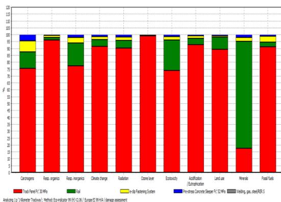
Figure 7 Damage Assessment of Railway Track
