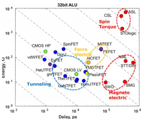
**Figure 4:** Energy switching versus delay of a 32-bit ALU
