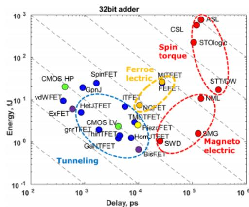
Figure 3: Switching energy versus delay of a 32-bit adder
