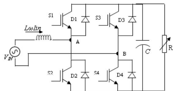
Fig. 1. Single-Phase full bridge converter.
