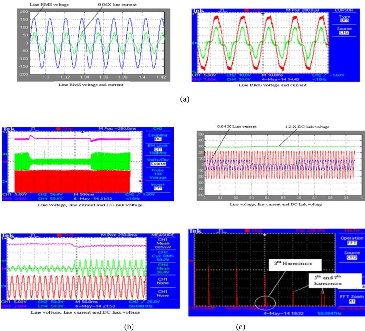
**Fig. 5.** (a) Simulation and experimental effects of line current and line voltage to indicate degraded power factor. (b) Simulated and experimental magnitudes of line voltage, line current and DC linked voltage when load changes from 80% to 5% intermittently to demonstrate distortions through voltage adjustment and equilibrium period. (c) Line current harmonics outline to indicate third, fifth and seventh harmonics are offered.
