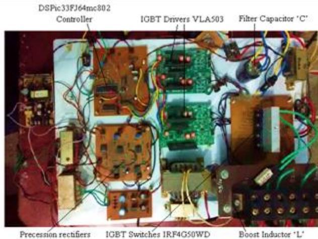
**Fig. 7:** Photograph of laboratory set-up.
