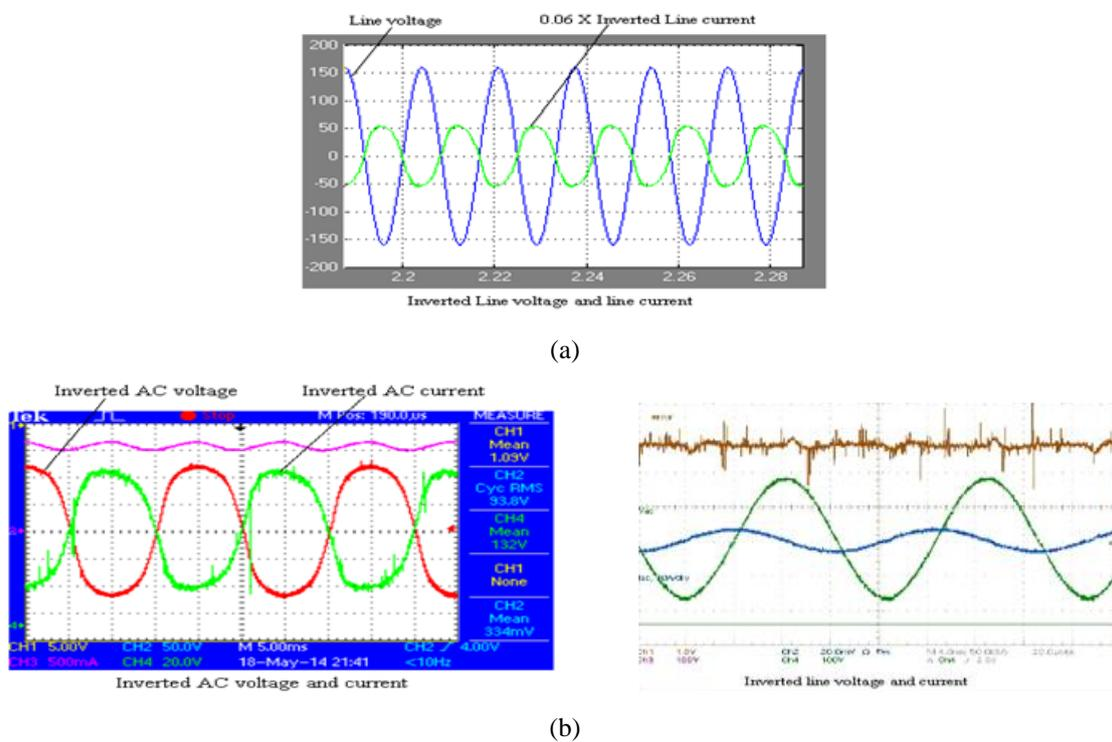
**Fig. 4.** (a) simulated values of reversed line current and line voltage at precisely 180° phase moved to demonstrate inversion activity (b) Experimental magnitudes of line voltage and line current for inductive load.
