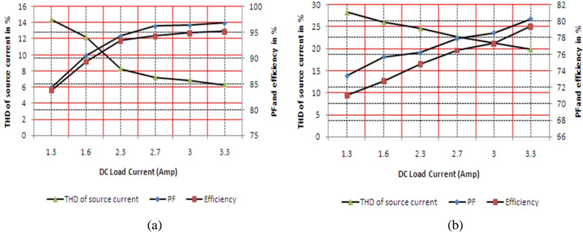
**Fig. 6.** (a) Variations in power factor, efficiency and total harmonics distortion with modification in load and DC load current for case I-rectification with CSPWM and inversion with SPWM. (b) Variations in power factor, efficiency and THD with modification in load and DC load current for case II-rectification and inversion both with SPWM.
