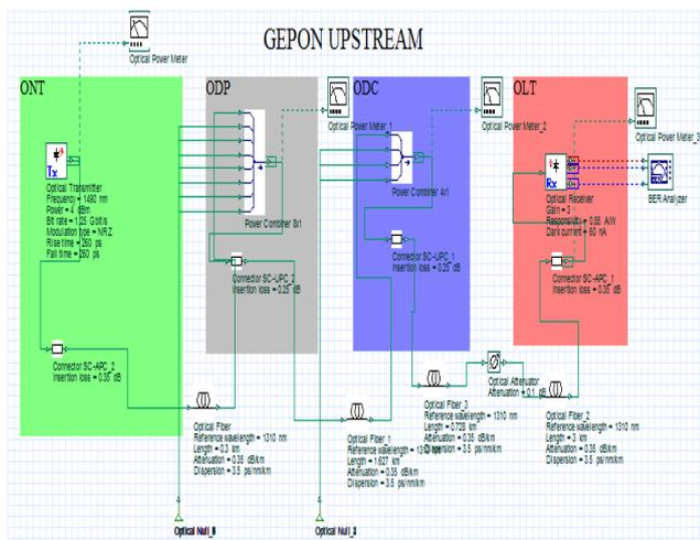
**Figure 6.** Upstream direction simulation using OptiSystem
