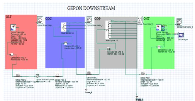
**Figure 3.** Downstream direction simulation using OptiSystem
