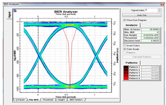
Figure 5. BER Analyzer for downstream direction simulation
