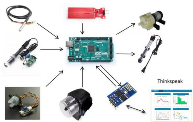
Fig 1. Block Diagram of smart aquaculture system
