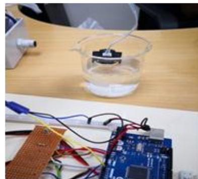
Fig 5. Implementing with turbidity sensor
