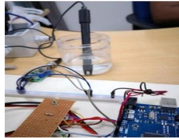
Fig 4. Implementing with pH sensor
