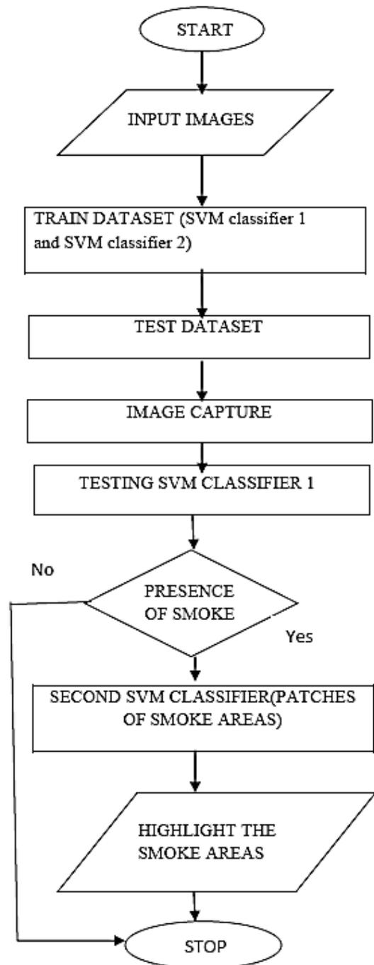
Figure 1. Proposed Smoke Detection technique
