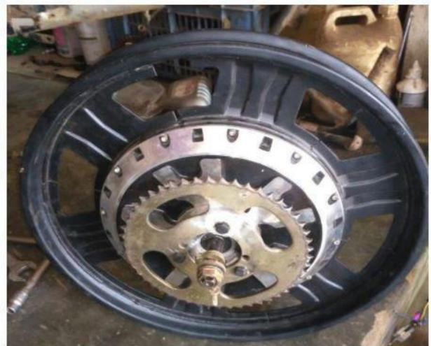
**Fig. 3.** Wheel Hub Motor with Chain Sprocket Assembly
