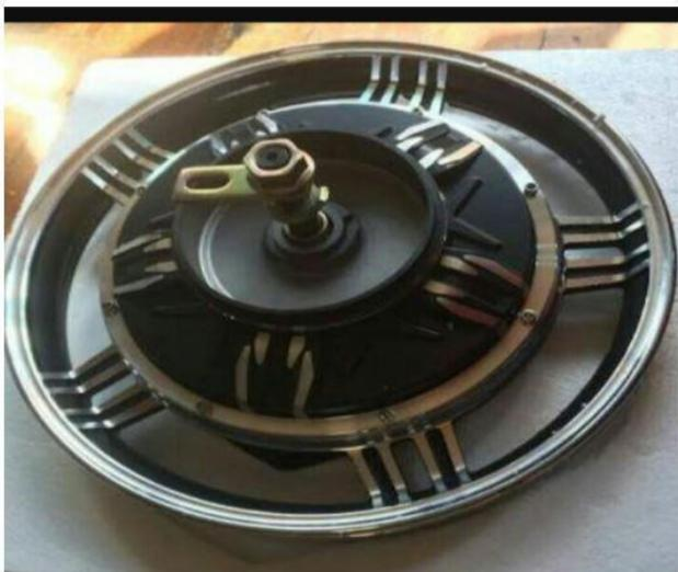
**Fig. 2.** Wheel Hub Motor without Chain Sprocket Assembly
