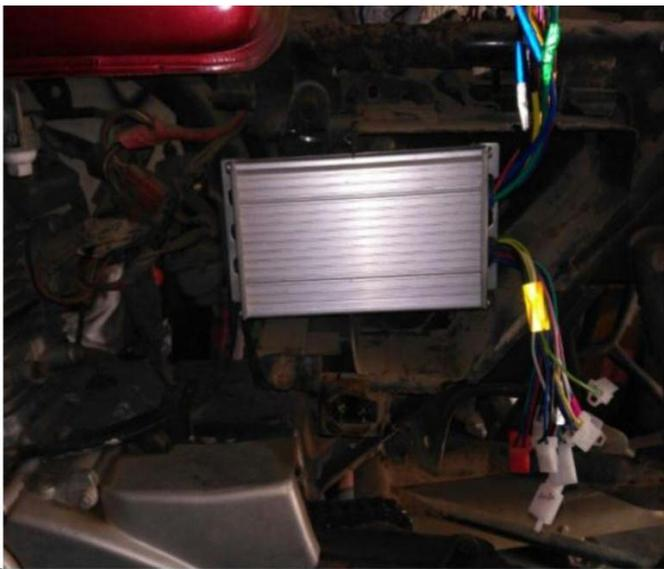
**Fig. 5.** Controller Position
