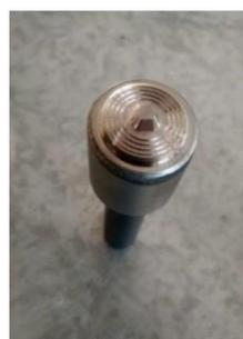
Fig 2.3: Photograph of FSP tool.
