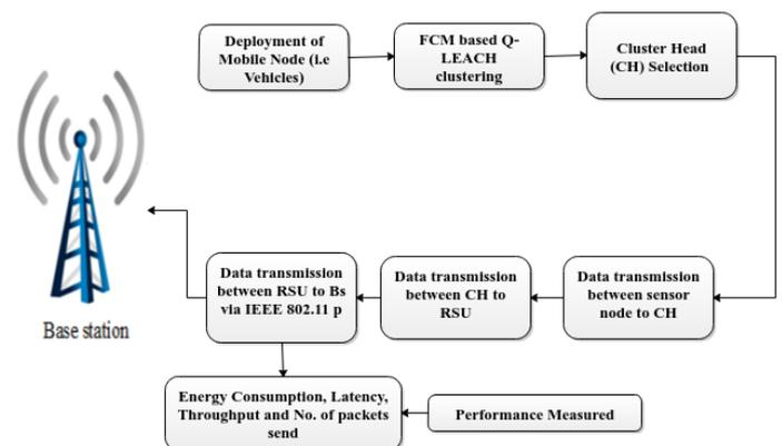
**Figure.1.** Block diagram of FCM-Q LEACH-VANET.
