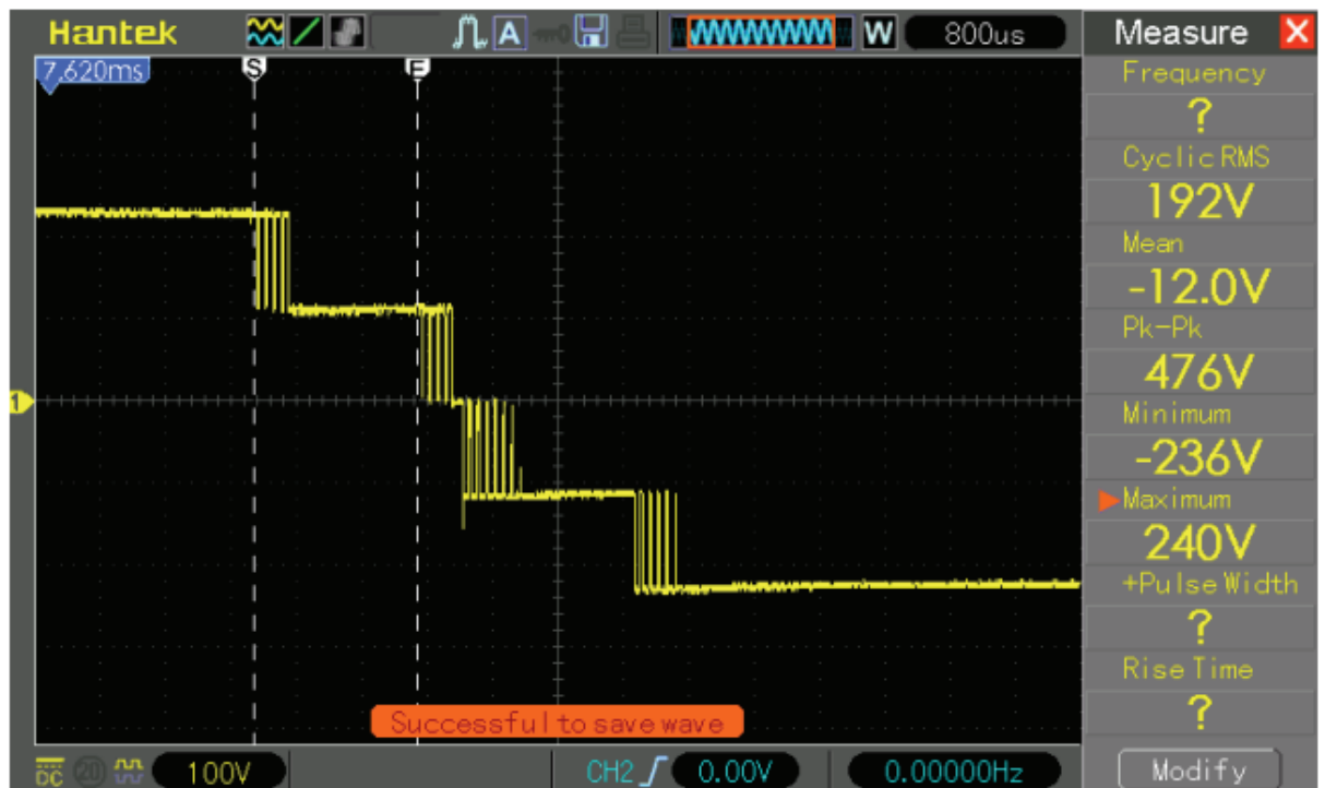
Figure 8. Voltage waveform of Five level generation with SPWM (Load 200W).
