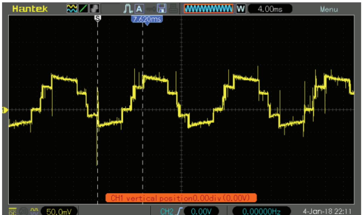
Figure 6. Current waveform of five level generation with SPWM (Load 100W).
