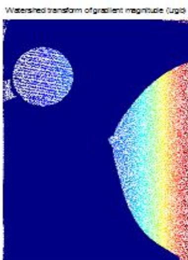
**Fig.2** Watershed transform of gradient Image
