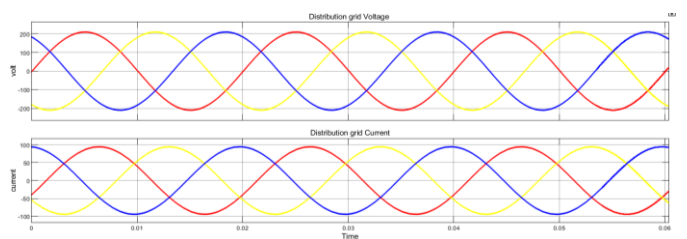
Fig. 17. Voltage and Current waveform of the proposed system at the grid side
