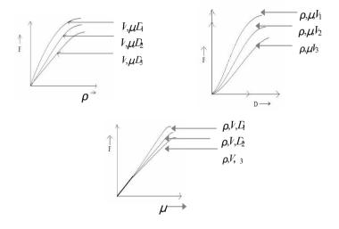
Dimensional less numbers are very needful. The number of parameters can be reduced by determining the proper dimensional less number for the flow. As it is seen that during calculation of drag for the flow about a sphere parameters are chosen V,  $\rho$ ,  $\mu$  and D. But with the help of non-dimensional numbers, we can get a relationship as follow,
