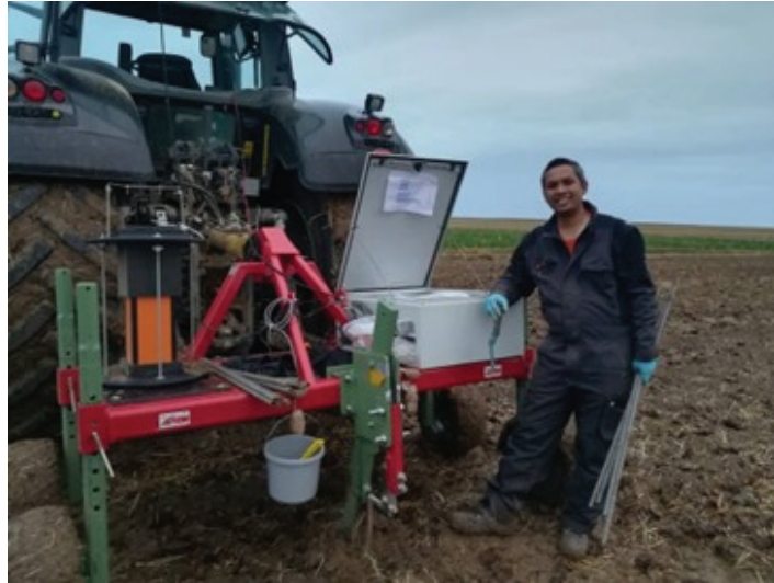
Figure 1. Shank that connected with load cell, optical sensor and gamma ray spectrometer
