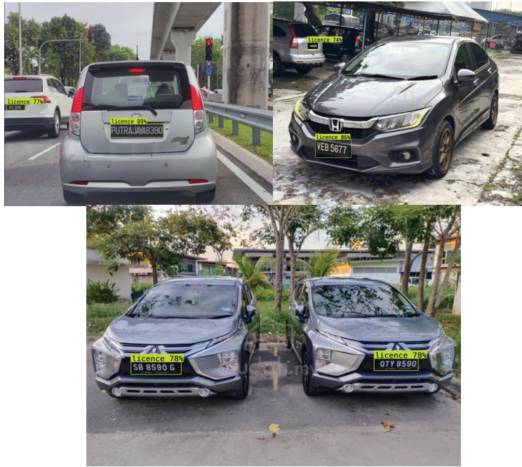
Figure 11: YOLOv8 license plate detection results demonstrating multi-vehicle and varying angle performance with the different confidence values
