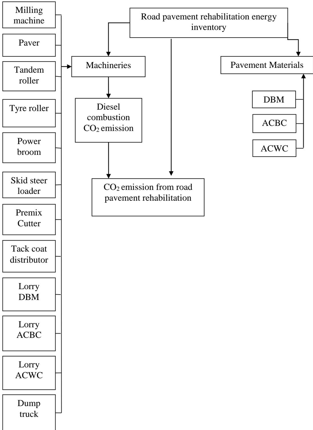
**Figure 2:** Framework of input and output adopted in the road pavement rehabilitation at Sungai Petani, Kedah
