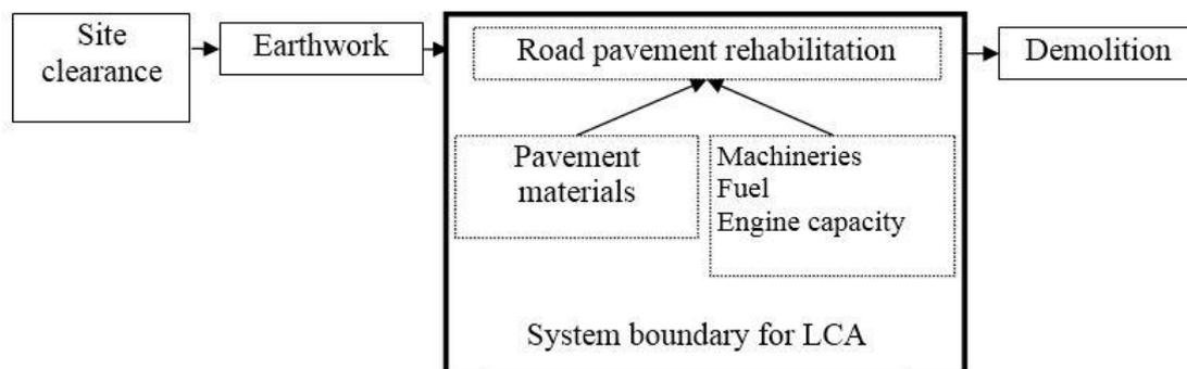
**Figure 1:** LCA system boundary for road pavement rehabilitation
