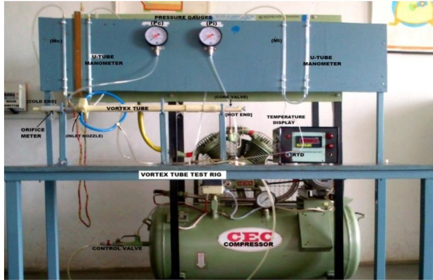
Fig. 2: Actual vortex tube experimental setup.
