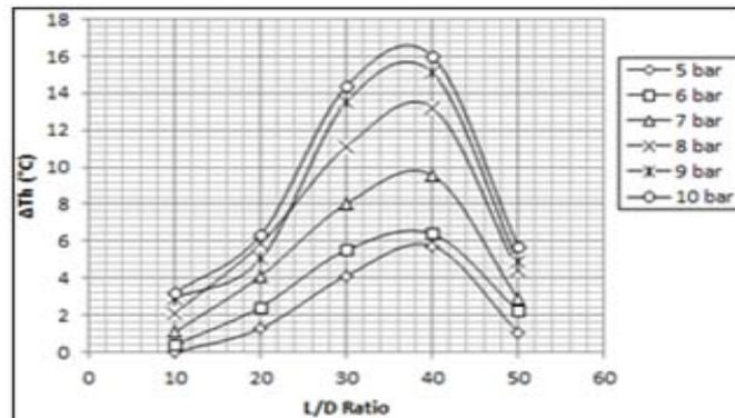
Fig. 4: The effect of L/D ratio on  $\Delta T_h$ .
