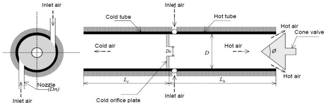
Fig. 1: Schematic diagram of counter-flow vortex tube [6].
