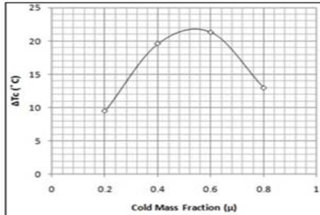
Fig. 5: The effect of cold mass fraction on  $\Delta T_c$ .
