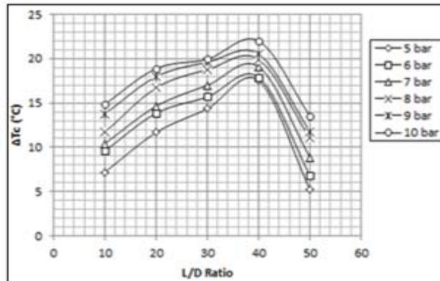
Fig. 3: The effect of L/D ratio on  $\Delta T_c$ .
