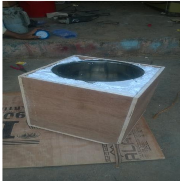
Figure 2: PCM container around the evaporator
