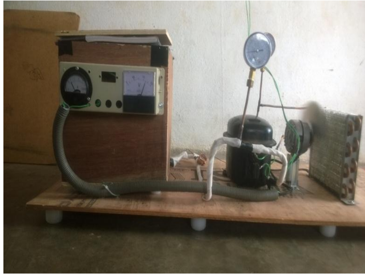
Figure 1: Vapour compression refrigeration test rig
